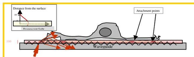
OWLS methods allow quantifying the deposition of material in a thin (<150 nm) layer above the solid sensor surface. In terms of cells, it can provide data on focal contacts and adhesion sites, while the rest of the cellular mass remains out of the field of detection.
