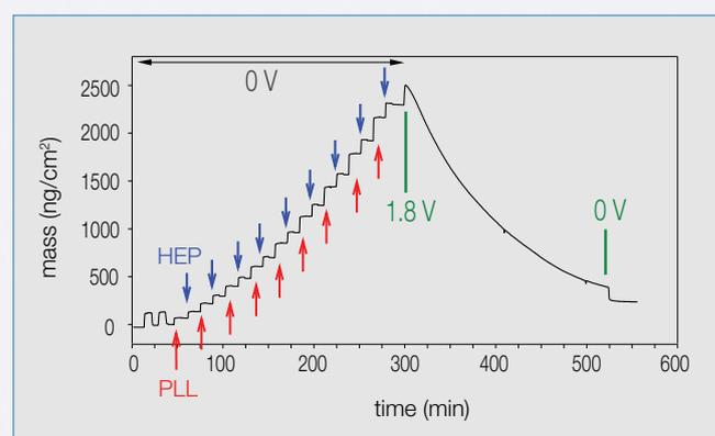
Build up of absorbed mass measured with EC-OWLS during the alternate deposition of PLL and HEP layers at an electrical potential of 0V. Application of 1.8V dissolves the polyelectrolyte layer as it is observed by the decrease of mass.
