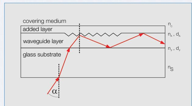
Supposing that  $N_{TE}$ ,  $N_{TM}$  have been calculated from the  $\alpha_{TE}$ ,  $\alpha_{TM}$  incoupling angles and the optical parameters of the waveguide layer ( $n_f, d_f$ ), of the substrate ( $n_s$ ), of the covering medium ( $n_c$ ) are known, the refractive index ( $n_a$ ), the thickness ( $d_a$ ) and the mass ( $M$ ) per area of the added layer can be determined.
