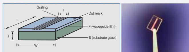
Grating: periodicity = 2400 lines/mm ( $0.4166 \mu\text{m}$ ); length (l)  $\sim 2$  mm
