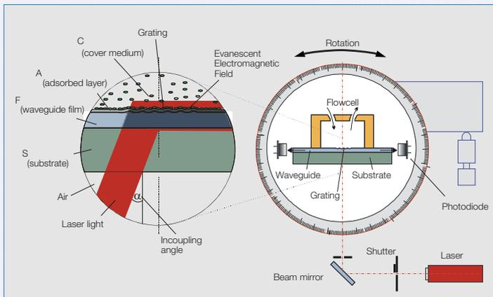
The basic principle of the OWLS method is that linearly polarized light (He-Ne laser) is coupled by a diffraction grating into the waveguide layer, provided that the incoupling condition is fulfilled.
