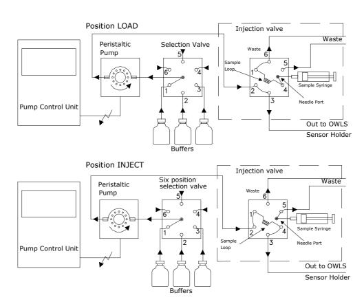
Model: OWLS SIS-03 (option) Stand Alone Sample Injection System with Peristaltic Pump
